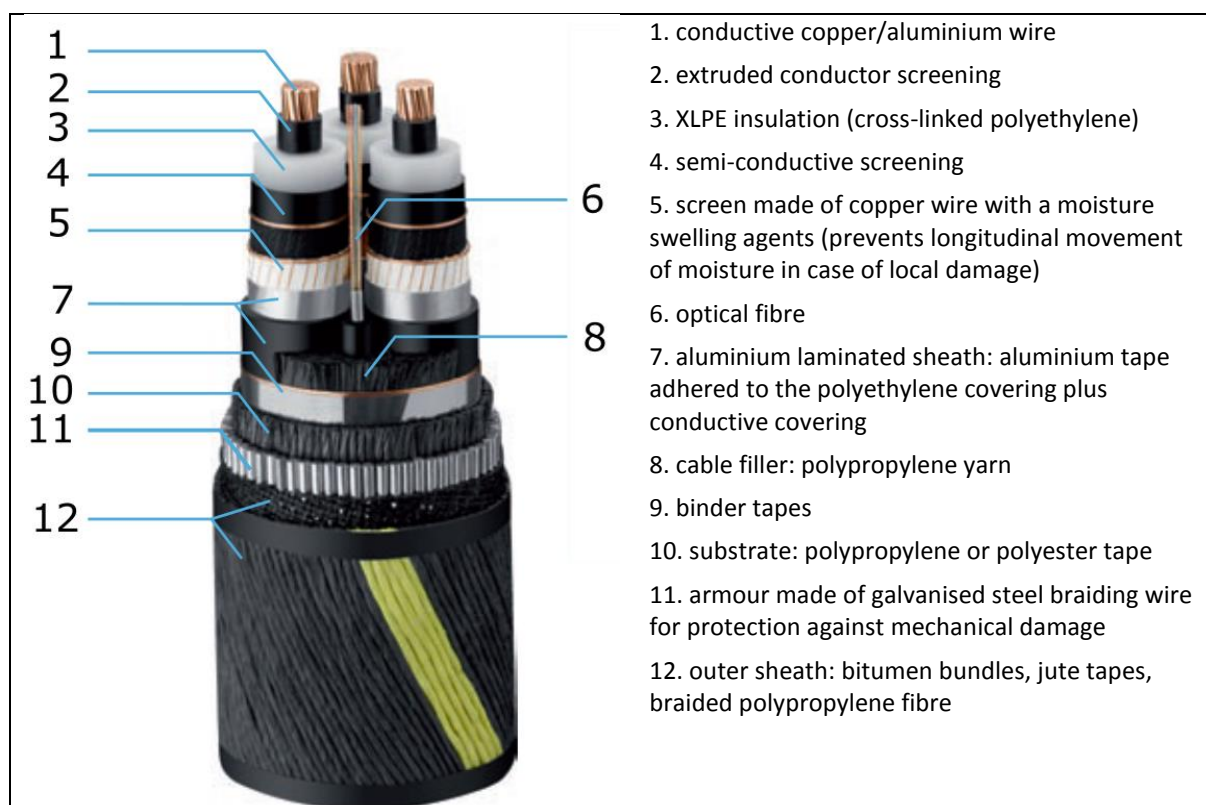
Figure 2.3. Construction of an exemplary extra high voltage subsea power cable [Source: internal materials on the basis of nexans.com]
